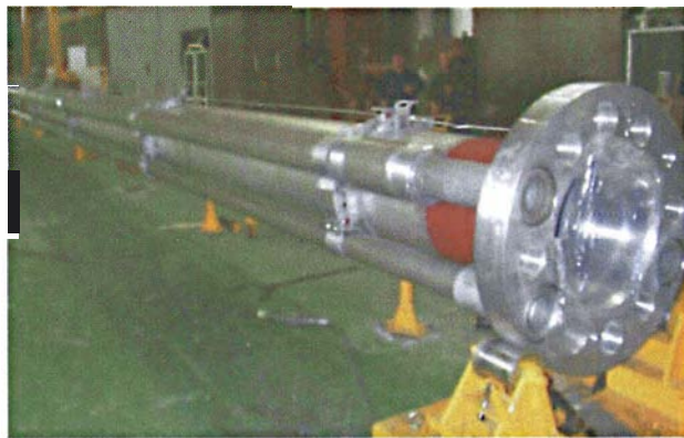
Noble Corp., with help from Aquatic, has developed lightweight aluminum riser for use in deepwater wells. (Photo courtesy of Noble Corp.)
