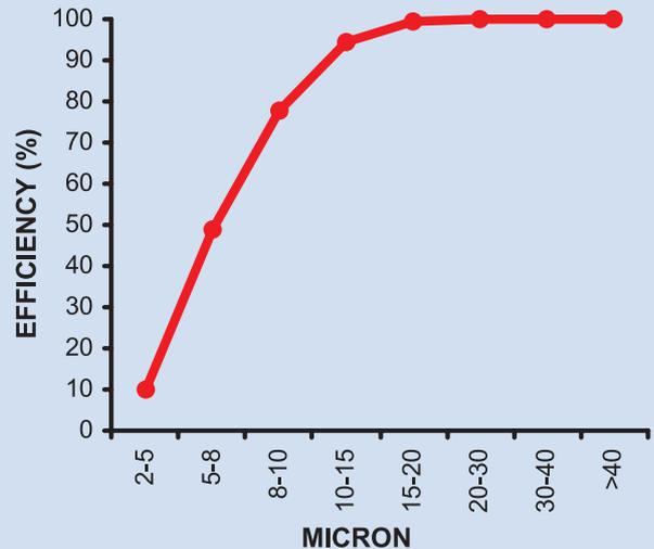
Test Method: Initial Efficiency ASTM F795-88
