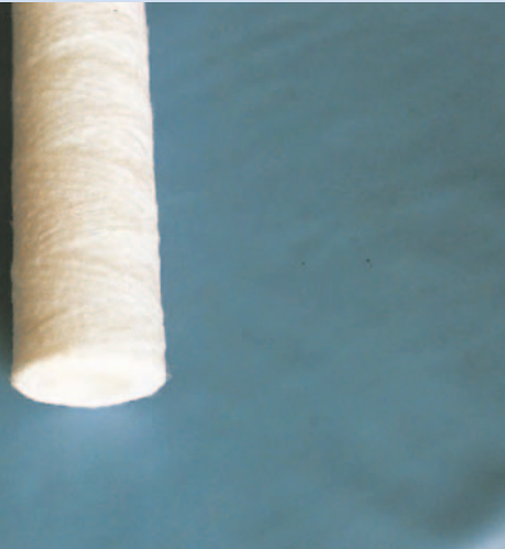
Figure 4: Cartridge made from continuous filament media.
